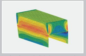
Simulation of stresses induced by breaking waves on a Dutch Floating Breakwater element (U-Block)
