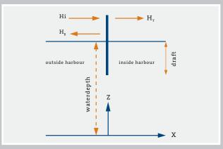
Incoming waveheight Hi, reflected waveheight Hr and transmitted waveheight Ht
