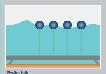
Balls are connected to the seabed by a flexible rod. Turbulant and and wave energy absorbing floating breakwater experiment.
