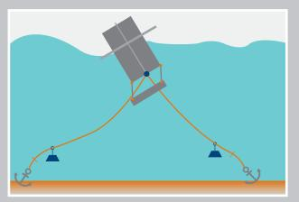
Wave barrier (steel structure with counter weight) Wave energy absorber and turbulant floating breakwater experiment.
